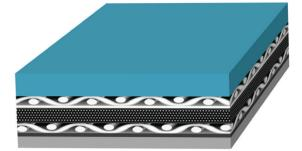
Strip 350 consists of an isotropic film carrier coated on one side with a specially formulated face compound developed for aqueous varnish systems, which can also be used for UV varnish systems. This special face compound exhibits extremely high mechanical strength (for increased longevity) facilitating perfect stripping even where profile angles are 25° or less.
